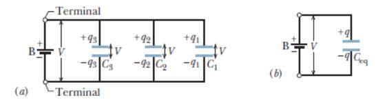
Figure b shows the equivalent capacitor (with equivalent capacitance  $C_{eq}$ ) that has replaced the three capacitors (with actual capacitances  $C_1, C_2$ , and  $C_3$ ) of Fig. a.
