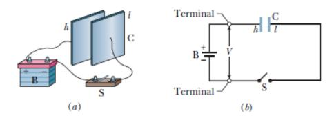
In Fig.a, a battery B, a switch S, an uncharged capacitor C, and interconnecting wires form a circuit.
