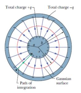
As a Gaussian surface, we choose a cylinder of length L and radius r, closed by end caps and placed as is shown in Fig. It is coaxial with the cylinders and encloses the central cylinder and thus also the charge q on that cylinder. Equation 2 then relates that charge and the field magnitude E as
