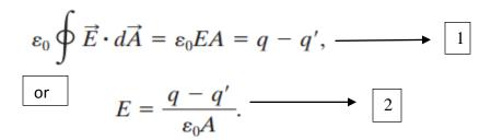
The effect of the dielectric is to weaken the original field  $E_0$  by a factor of k; so we may write
