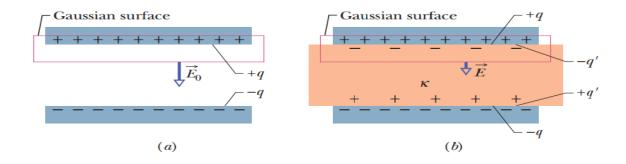
**Fig 1.** A parallel-plate capacitor (a) without and (b) with a dielectric slab inserted. The charge q on the plates is assumed to be the same in both cases.
