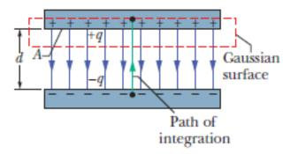
We draw a Gaussian surface that encloses just the charge q on the positive plate, as in above Fig.. From Eq. 2 we can then write
